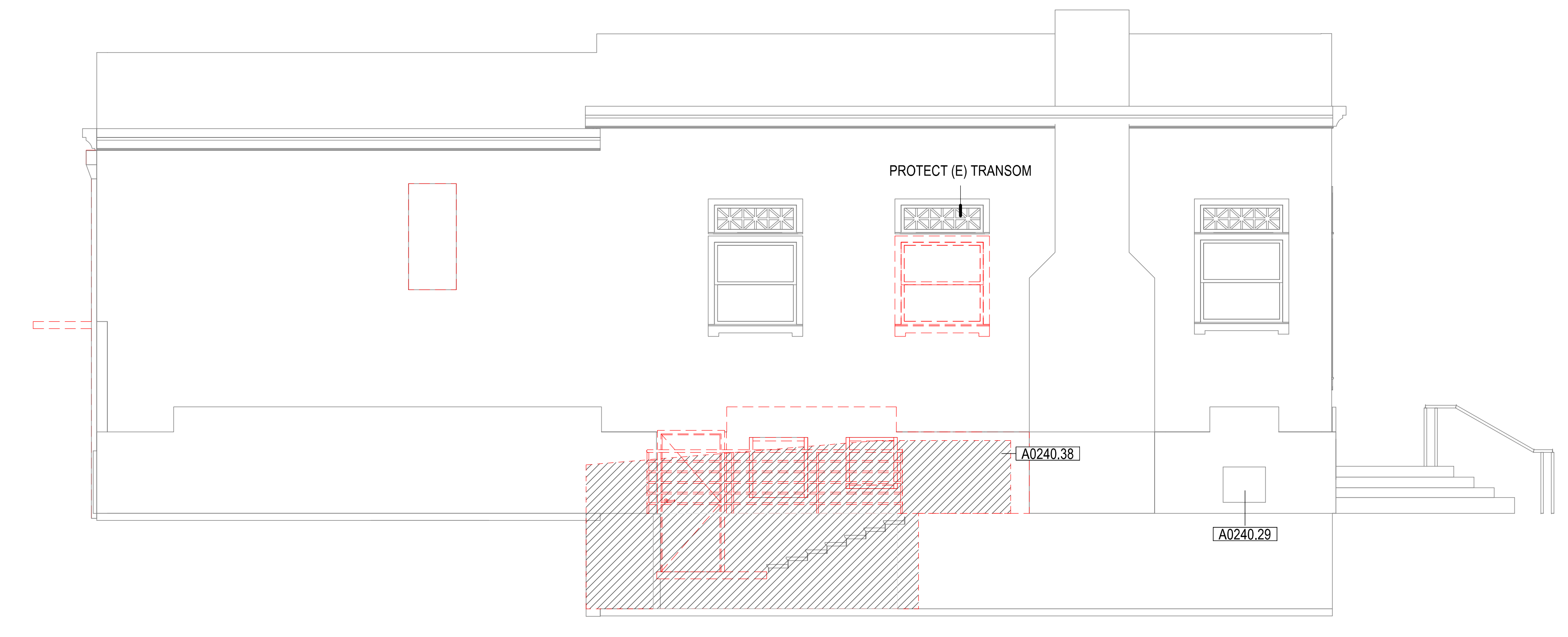
1 BUILDING ELEVATION - WEST WALL (E) STUCCO DEMOLITION 1/4" = 1'-0"
